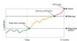
Logged data from a turbine vs time. Diagnostic models enable advice to be issued well before the turbine generates a warning or an alarm, allowing timely advance planning of appropriate service activities
